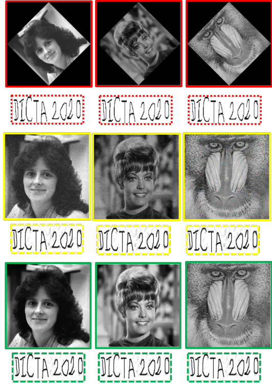
Fig. 5. Robustness/Security comparisons of the proposed scheme. Solid red, yellow and green boundaries contain the watermarked images under rotation attack at 45^\circ , Gaussian Noise at 0.001 and JPEG compression (QF=40), respectively. All dashed boundaries represent the extracted watermarks from the attacked watermarked images. Best viewed when zoomed in.
