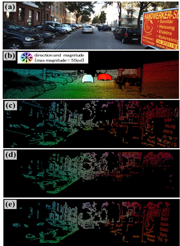
Fig. 6: Result of motion parallax estimation. (a)input image, (b)ground truth, (c)Tarrío et al[9], (d)Ramalingam et al[8], and (e)our method.
